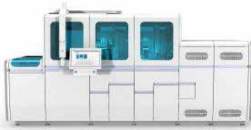
**Cobas 8800 Analyser – The high throughput platform consists of a sample handling unit, extraction compartment and a separate isolated amplification compartment. Reagents are ready to use and can be stored on-board in a refrigerated unit for up to 30 days**
